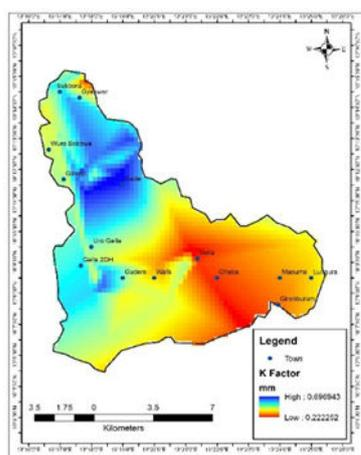
**Figure 7:** Soil Erodibility Factor (K-Factor). Source: Author's Analysis.
