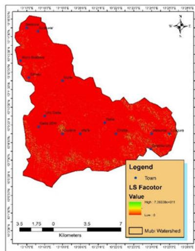
**Figure 8:** Slope Length and Steepness (LS-Factor). Source: Author's Analysis.
