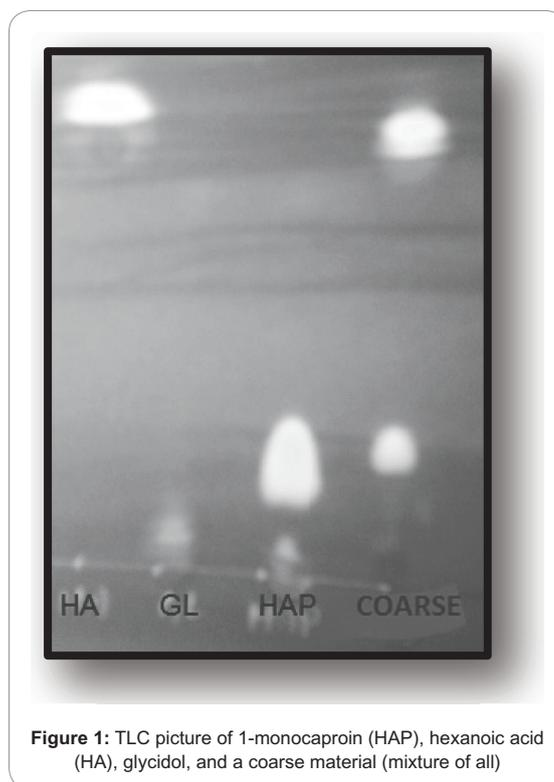
Figure 1: TLC picture of 1-monocaproin (HAP), hexanoic acid (HA), glycidol, and a coarse material (mixture of all)
