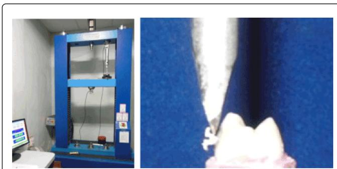
**Figure 3:** (a) Universal testing machine, (b) Premolar with bracket bonded and the chisel tip acting in the upper part of the bracket base during shear bond strength test
