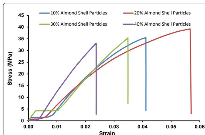
Figure 5b: Stress-strain diagram for different wt% of almond particle with 1.0 wt% of depolymerised natural rubber.
