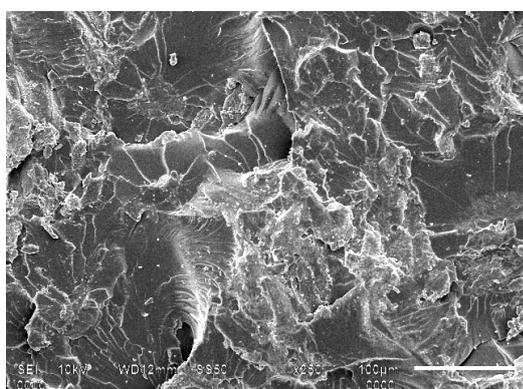
Figure 10c: Scanning electron micrograph of 1 wt% DNR & 20 wt% almond shell particles composite material at magnification 250x.
