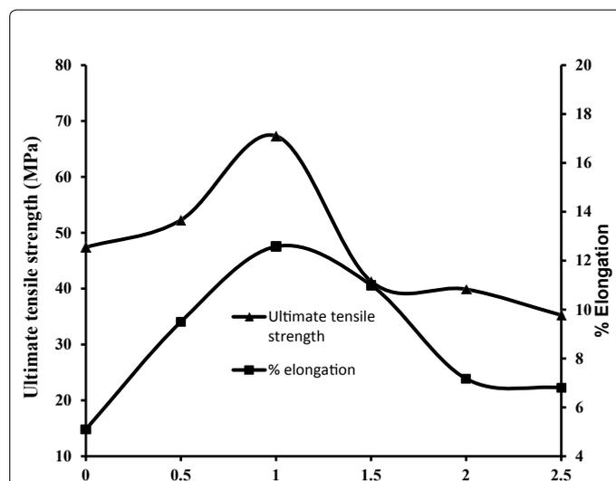
Figure 5c: Effect of wt% DNR on ultimate tensile strength and % elongation.
