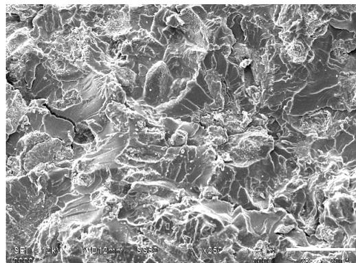
Figure 10e: Scanning electron micrograph of 1 wt% DNR & 40 wt% almond shell particles composite material at magnification 250x.
