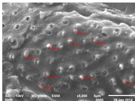
Figure 10f: Scanning electron micrograph of 1 wt% DNR & 30 wt% almond shell particles composite material at magnification 5000x.
