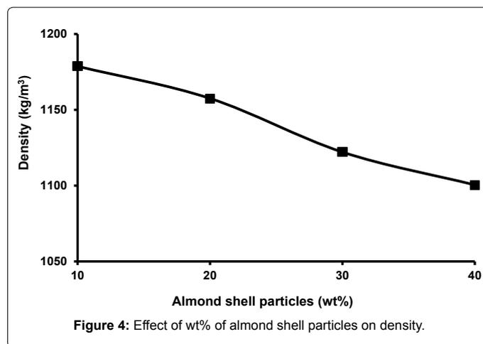
Figure 4: Effect of wt% of almond shell particles on density.
