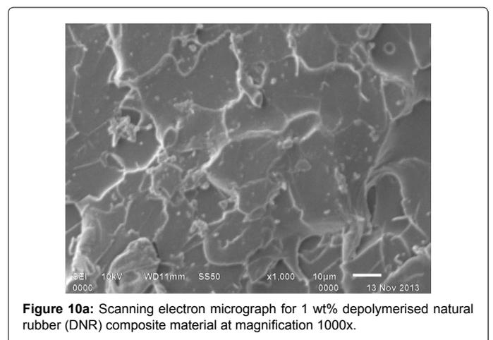
in epoxy resin. Good crosslinking of DNR with epoxy resin can be seen here leads to enhanced mechanical properties as this crosslinking overcome the brittle behaviour of epoxy resin.
