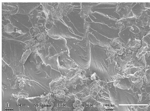
Figure 10b: Scanning electron micrograph of 1 wt% DNR & 10 wt% almond shell particles composite material at magnification 250x.
