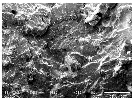
Figure 10d: Scanning electron micrograph of 1 wt% DNR & 30 wt% almond shell particles composite material at magnification 250x.
