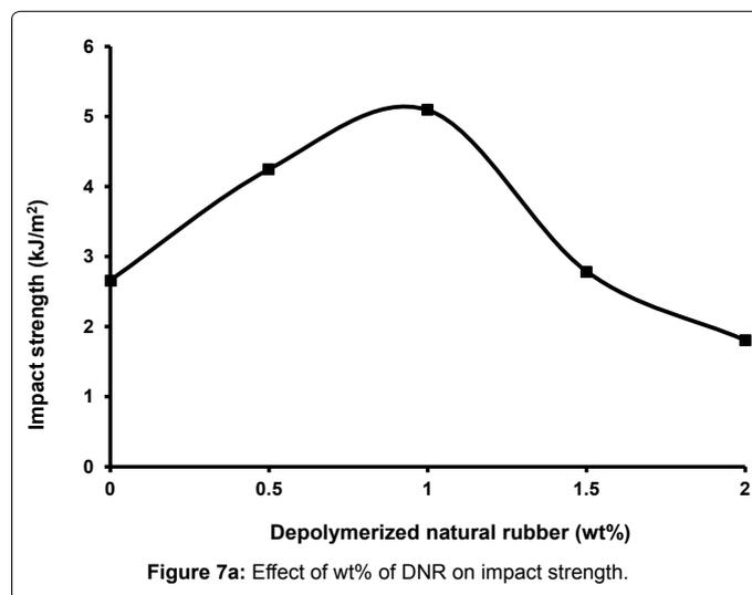
The results show that by adding DNR in epoxy resin the impact strength of epoxy resin is increased by 80% on 1 wt% of DNR which is a very remarkable improvement. As Chuayjuljit [3] concluded that ENR product was applied as impact modifier for epoxy resin and Kumar and Kothandaraman [5] modified epoxy resin with maleate
