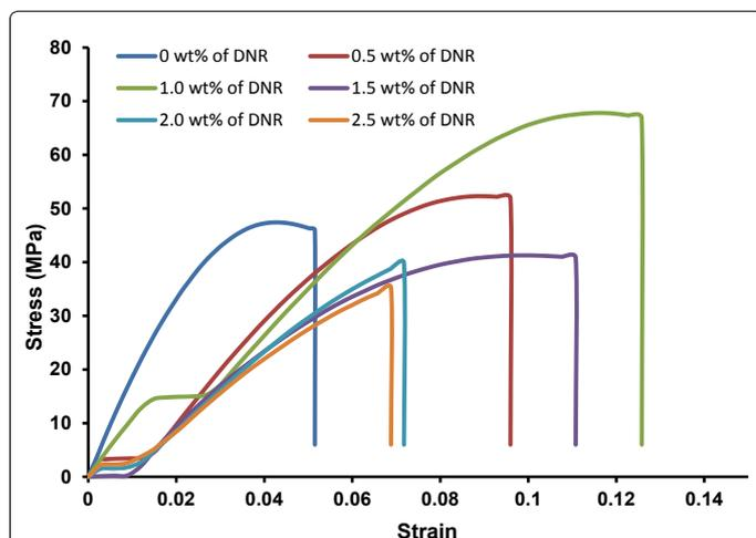
Figure 5a: Stress-strain diagram for different wt% of depolymerised natural rubber (DNR).
