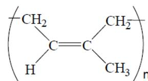
**Figure 2:** Chemical structure of *cis* 1, 4-polyisoprene.
