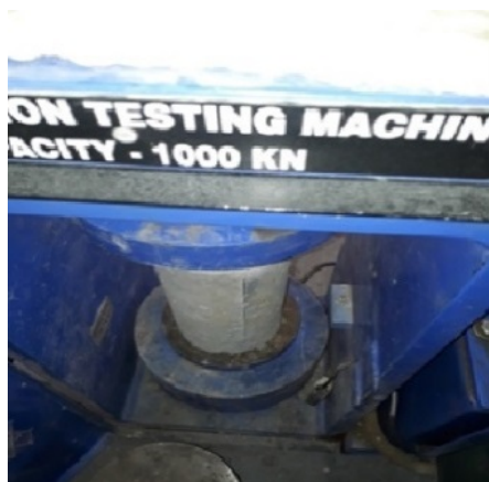
Figure 3: Testing of circular column on CTM.
