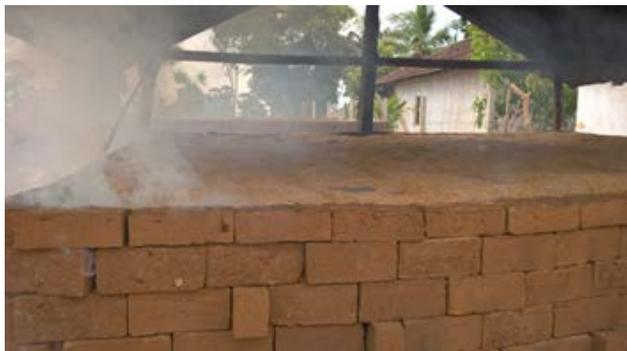
Figure 4: Traditional firing method of clay bricks.
