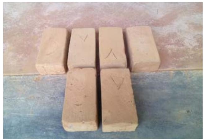
Figure 3: Sri Lankan standard brick size: 20.5 cm × 9.5 cm × 7.5 cm.
