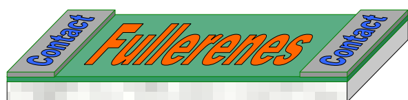
Figure 1: Illustration of the set up device obtained from a substrate of glass with gold contacts on both sides. The gold contacts were directly connected to the electrometer to collect V/I characteristics of fullerenes C_{60} nanoassembled.
