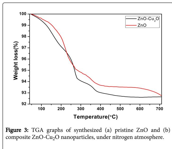
Figure 3: TGA graphs of synthesized (a) pristine ZnO and (b) composite ZnO-Cu<sub>2</sub>O nanoparticles, under nitrogen atmosphere.
