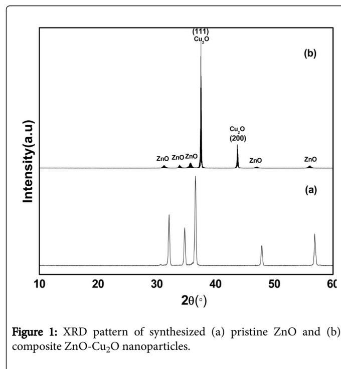
Figure 1: XRD pattern of synthesized (a) pristine ZnO and (b) composite ZnO-Cu<sub>2</sub>O nanoparticles.
