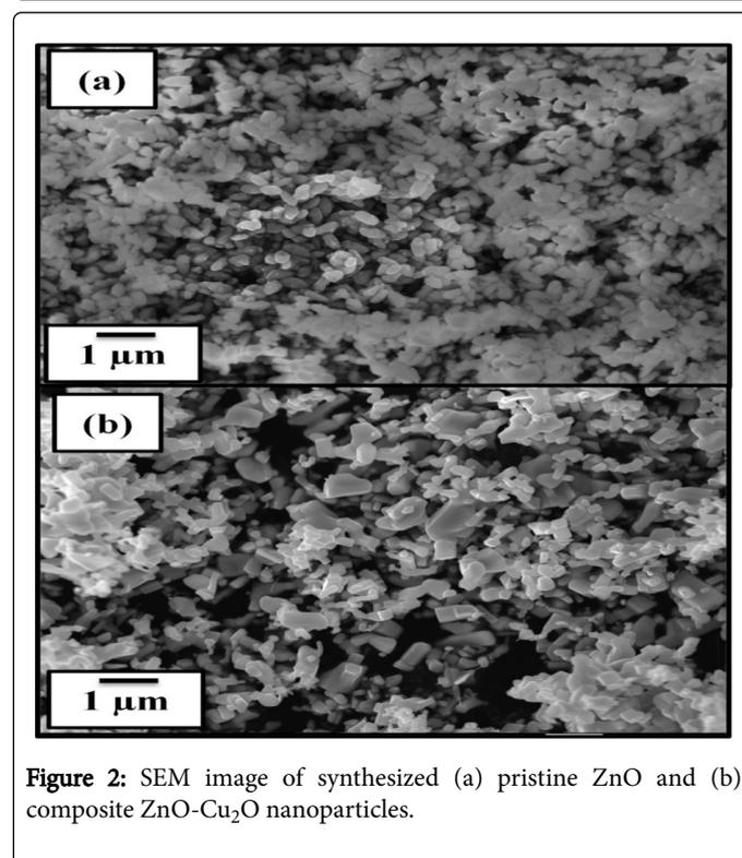
Figure 2: SEM image of synthesized (a) pristine ZnO and (b) composite ZnO-Cu<sub>2</sub>O nanoparticles.
