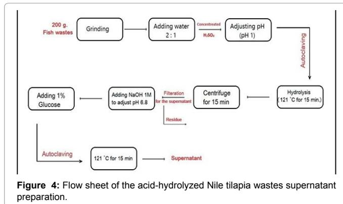
Figure 4: Flow sheet of the acid-hydrolyzed Nile tilapia wastes supernatant preparation.
