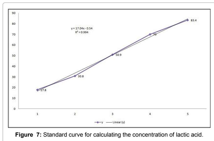
Figure 7: Standard curve for calculating the concentration of lactic acid.
