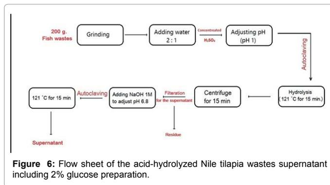
Figure 6: Flow sheet of the acid-hydrolyzed Nile tilapia wastes supernatant including 2% glucose preparation.
