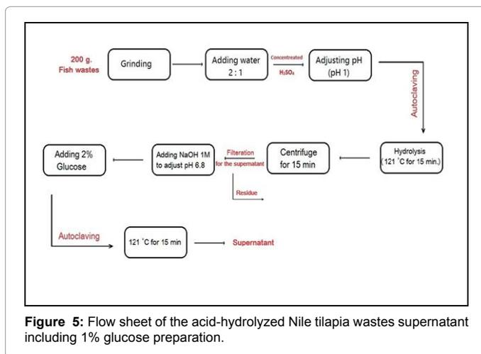
Figure 5: Flow sheet of the acid-hydrolyzed Nile tilapia wastes supernatant including 1% glucose preparation.
