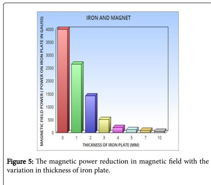
Figure 5: The magnetic power reduction in magnetic field with the variation in thickness of iron plate.
