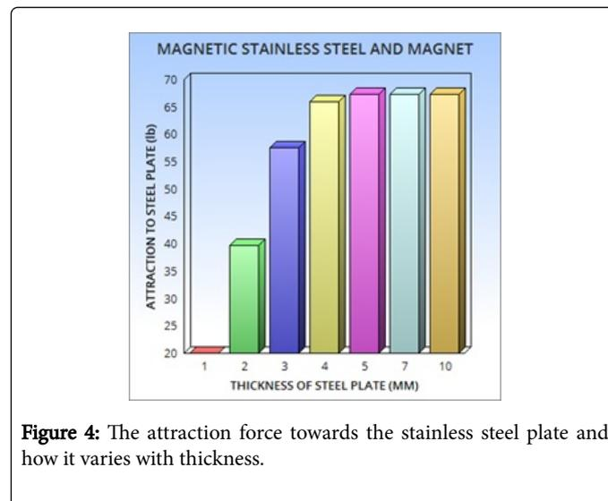
Figure 4: The attraction force towards the stainless steel plate and how it varies with thickness.
