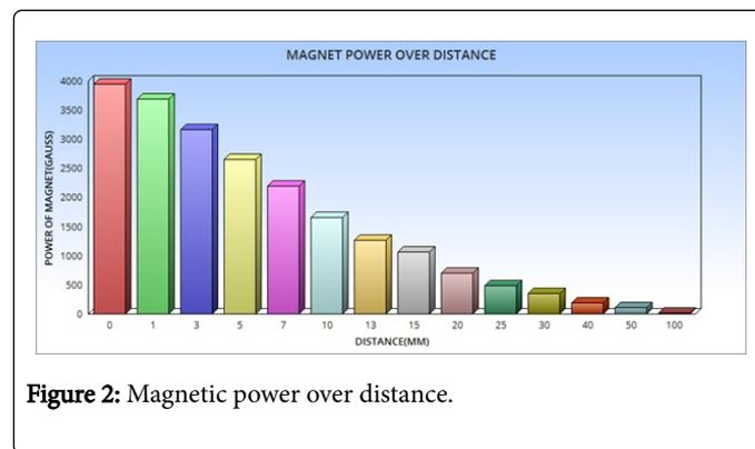
Figure 2: Magnetic power over distance.
