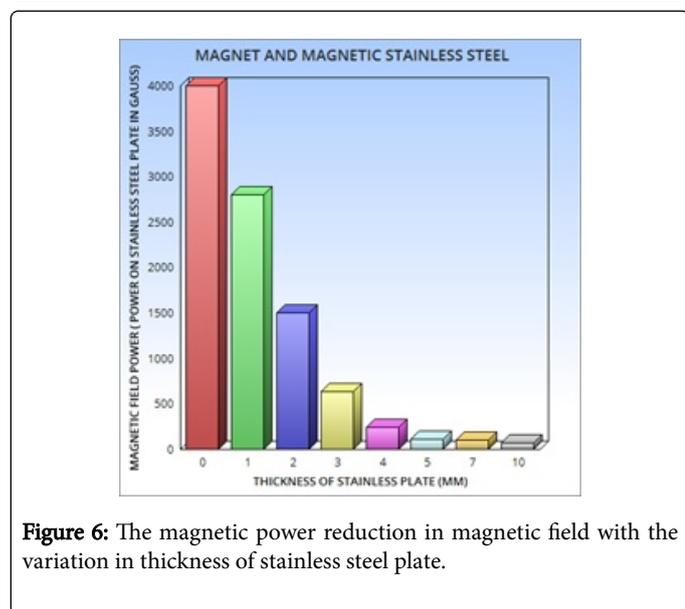
Figure 6: The magnetic power reduction in magnetic field with the variation in thickness of stainless steel plate.
