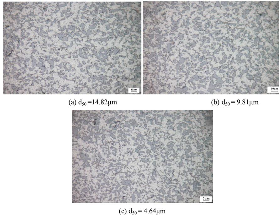
Figure 5: Influence of median particle size on microstructure of Al-50Si compounds.
