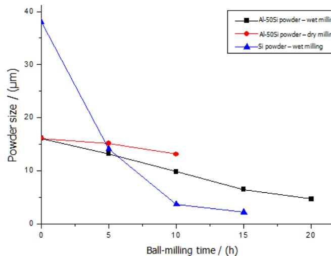
Figure 4: Relation between ball-milling time and particle size.
