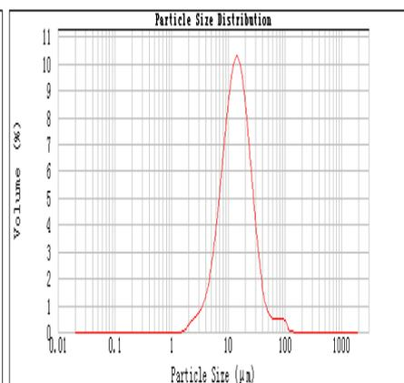
(b) dry ball-milling ( $d_{50}=15.10\mu\text{m}$ )
