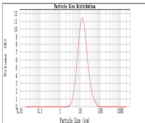
(a) wet ball-milling ( $d_{50}=13.19\mu\text{m}$ )
