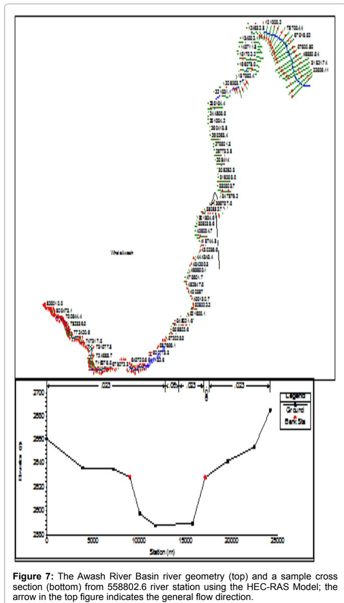
Figure 7: The Awash River Basin river geometry (top) and a sample cross section (bottom) from 558802.6 river station using the HEC-RAS Model; the arrow in the top figure indicates the general flow direction.
