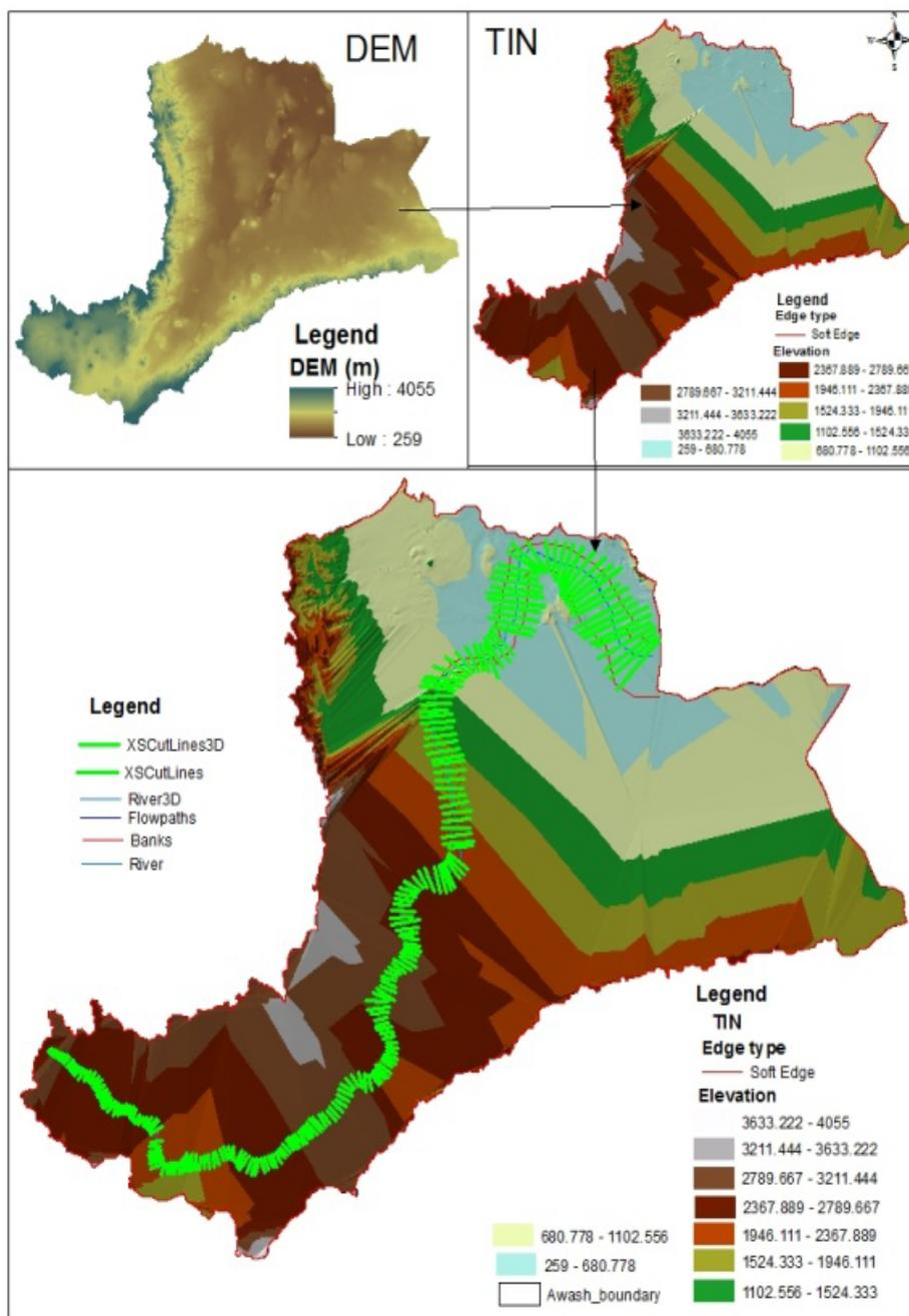
Figure 6: The Awash River Basin geometry data preparation using HEC-GeoRAS.
