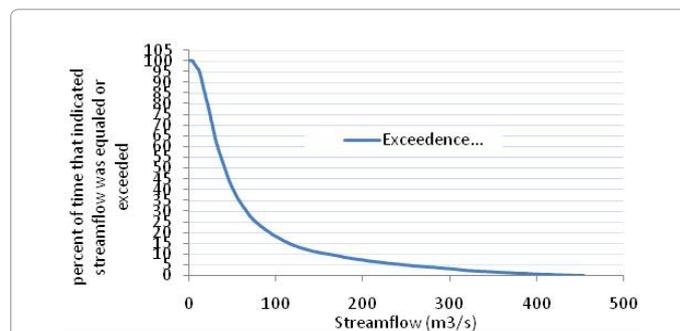
Figure 8: Daily mean flow frequency duration curve for the Awash River Basin at Dubti gauging station.
