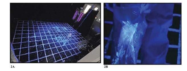
Figure 2: Use of fluorochromes to investigate spread of projectile vomiting. 2A) Shows splash and droplet dispersal in a test chamber after simulated projectile vomiting. 2B) Shows cross contamination on clothing of person undertaking clean-up.
