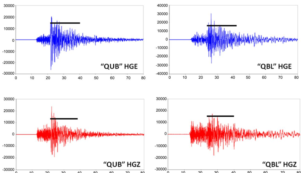
**Figure 4:** The horizontal and vertical components of the seismic signal on stations «QUB» and «QBL».
