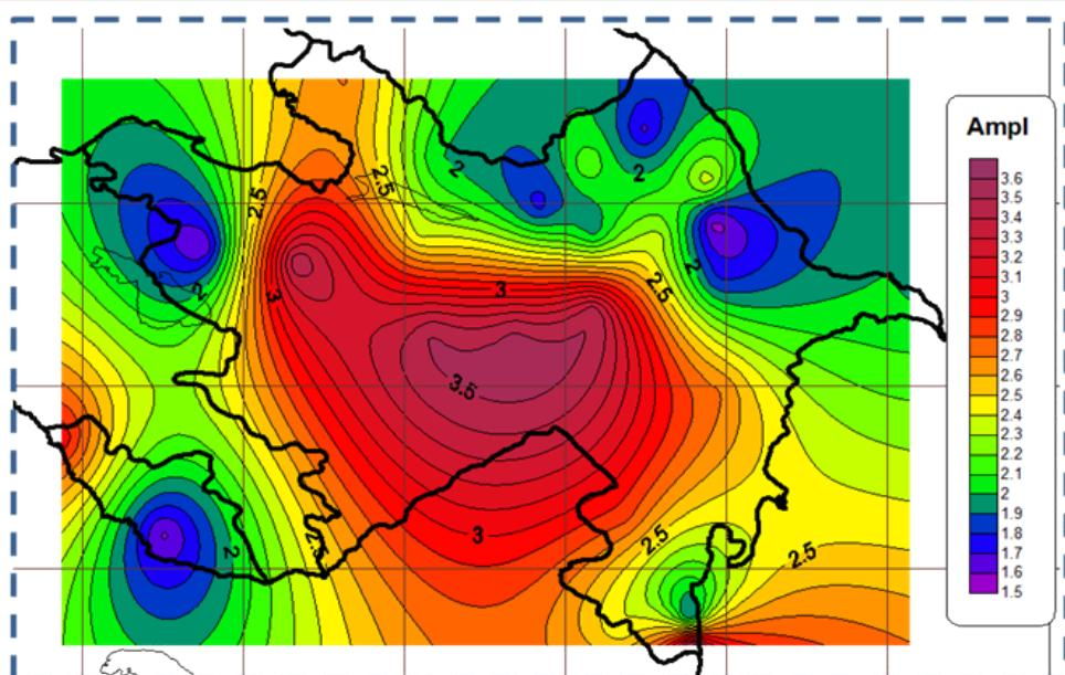
Figure 8: A distribution map of amplification factor of the transverse seismic waves on the digital stations, according to the data of strong earthquakes occurred in the years 2005-2015.
