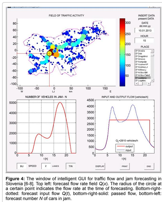
Figure 4: The window of intelligent GUI for traffic flow and jam forecasting in Slovenia [6-8]. Top left: forecast flow rate field  $Q(x)$ . The radius of the circle at a certain point indicates the flow rate at the time of forecasting. Bottom-right-dotted: forecast input flow  $Q(t)$ , bottom-right-solid: passed flow, bottom-left: forecast number  $N$  of cars in jam.
