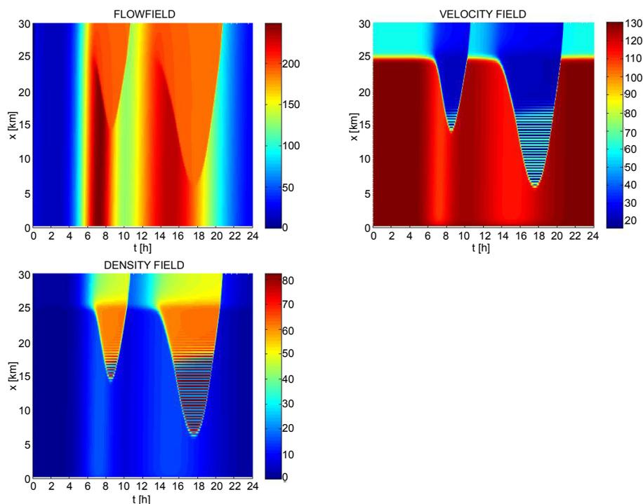
Figure 9a: Distributions of traffic field variables shown in ground plan: top-flow rate, middle-velocity, bottom-density.
