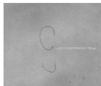
Figure 2: Showing point of intersection Ink of exhibit 1 shows absorption at 725 nm however ink of exhibit 2 does not show any absorption up to 778 nm.
