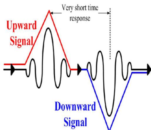
**Figure 2:** Transient signals induced by the energy violation.
