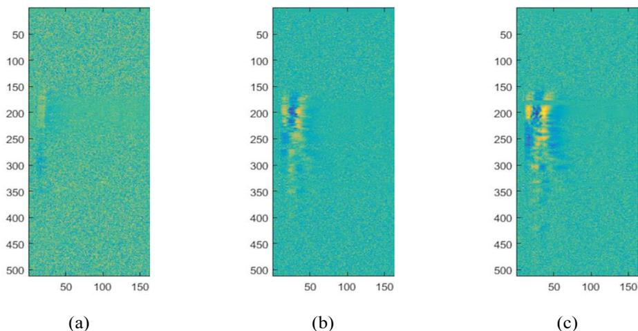
**Figure 5:** Wave propagation pattern inside tissue phantom for (a) 6 (b) 7 and (c) 8 mJ of pumping energy.
