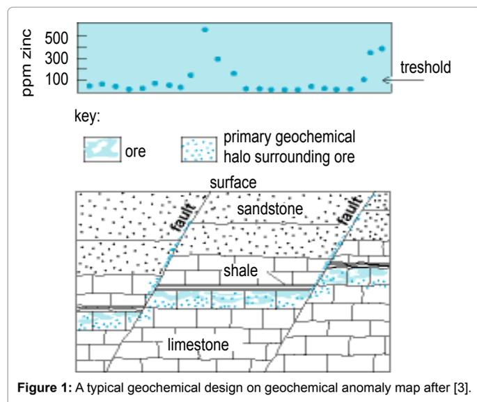
Figure 1: A typical geochemical design on geochemical anomaly map after [3].
