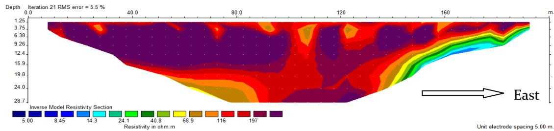
**Fig 6.** Wenner inverse model of line A002.
