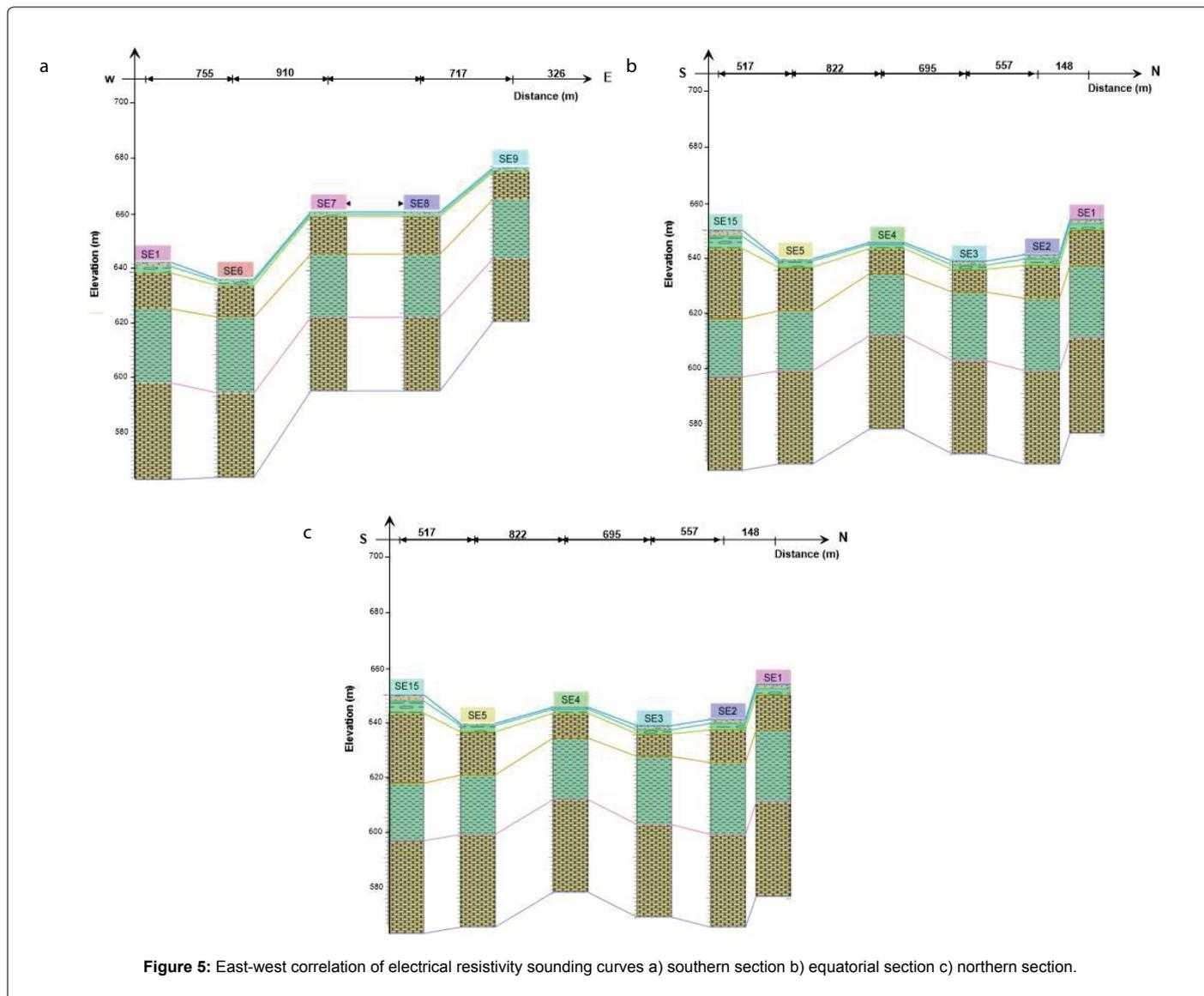
**Figure 5:** East-west correlation of electrical resistivity sounding curves a) southern section b) equatorial section c) northern section.
