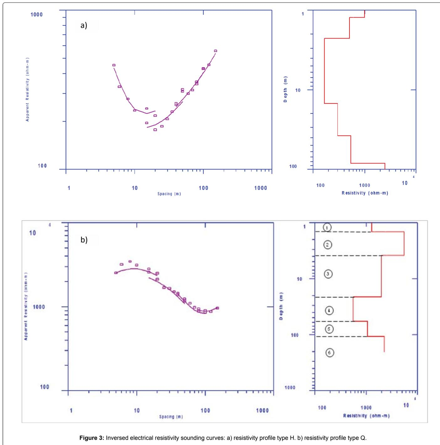
Figure 3: Inversed electrical resistivity sounding curves: a) resistivity profile type H. b) resistivity profile type Q.
