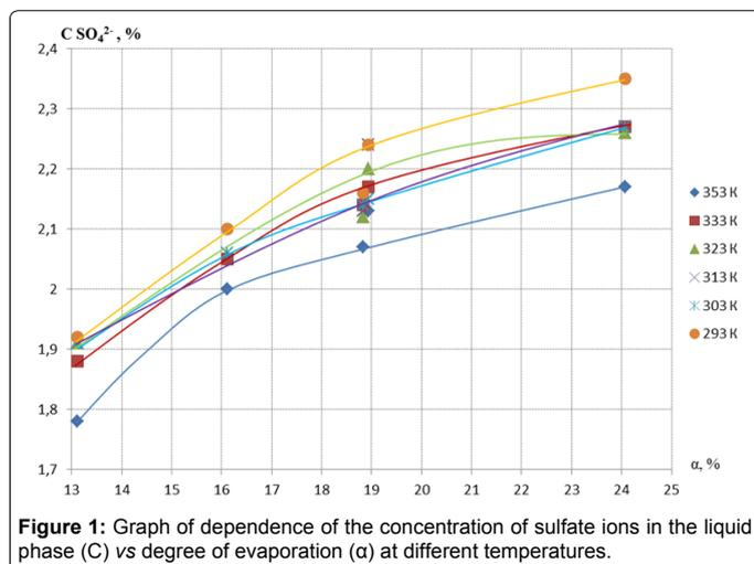
Figure 1: Graph of dependence of the concentration of sulfate ions in the liquid phase (C) vs degree of evaporation (α) at different temperatures.
