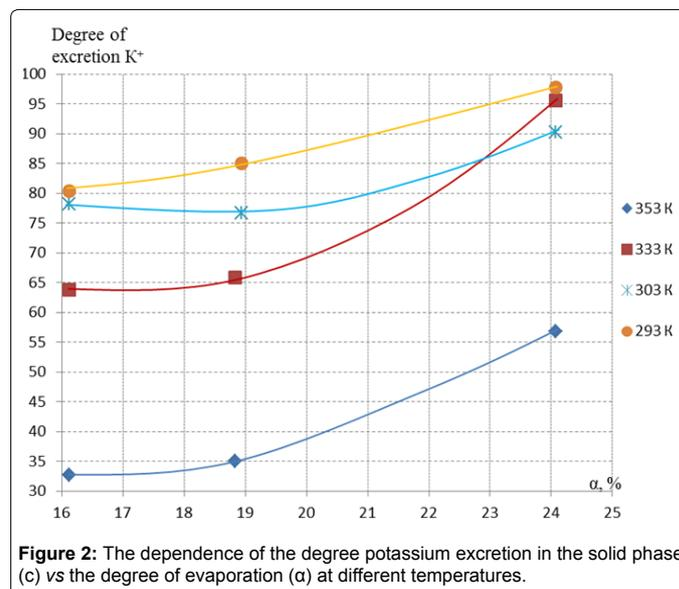
Figure 2: The dependence of the degree potassium excretion in the solid phase (c) vs the degree of evaporation (α) at different temperatures.
