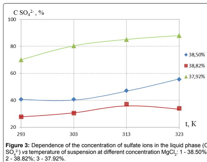
Figure 3: Dependence of the concentration of sulfate ions in the liquid phase ( $C SO_4^{2-}$ , %) vs temperature of suspension at different concentration  $MgCl_2$ : 1 - 38.50%; 2 - 38.82%; 3 - 37.92%.
