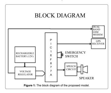
interfaced with all the other modules of the device. The program for PIC microcontroller is done in Embedded C language and is dumped using a kit.
