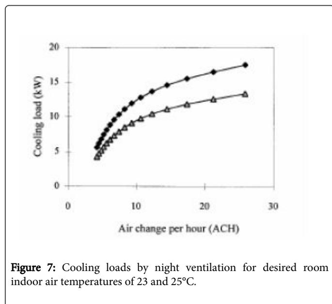
**Figure 7:** Cooling loads by night ventilation for desired room indoor air temperatures of 23 and 25°C.
