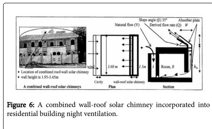
**Figure 6:** A combined wall-roof solar chimney incorporated into residential building night ventilation.
