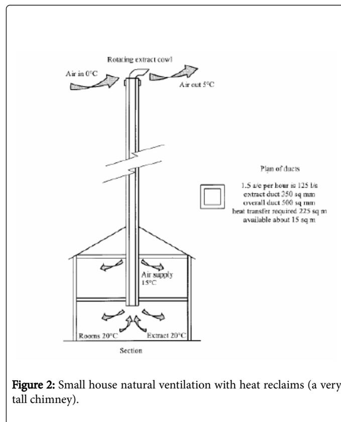
Figure 2: Small house natural ventilation with heat reclaims (a very tall chimney).
