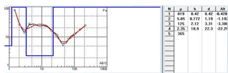
Figure 8: Resistivity Variation curve of VES Point 2.
