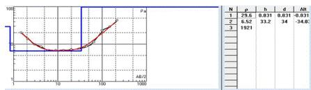
Figure 7: Resistivity variation curve of VES point 1.
