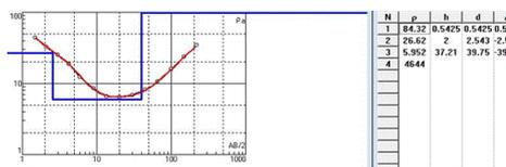
Figure 11: Resistivity Variation curve of VES Point 5.
