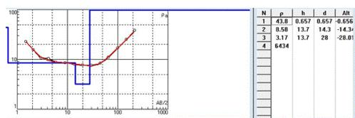
Figure 12: Resistivity Variation curve of VES Point 6.
