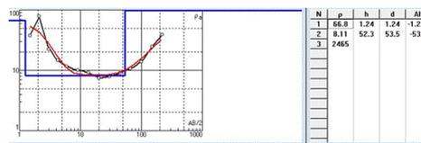
Figure 10: Resistivity Variation curve of VES Point 4.
