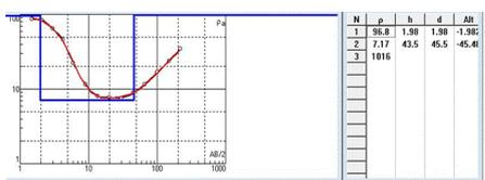
Figure 9: Resistivity Variation curve of VES Point 3.
