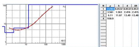
Figure 14: Resistivity Variation curve of VES Point 8.
