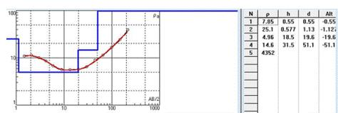
Figure 13: Resistivity Variation curve of VES Point 7.
