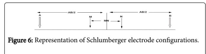
Figure 6: Representation of Schlumberger electrode configurations.
