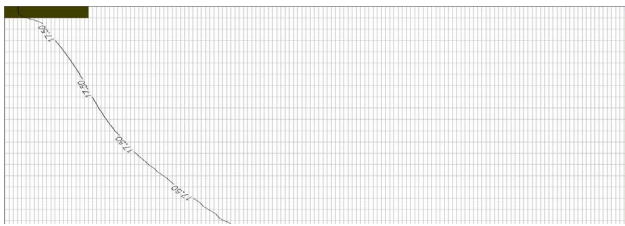
Figure 8: Seawater-freshwater interface location (at 50% of the maximum concentration) of case-2.
