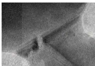
Figure 4: Particle binds totally to the bulk at time: t=780 seconds (binding contact area is about 50\text{ nm} \times 50\text{ nm} ).
