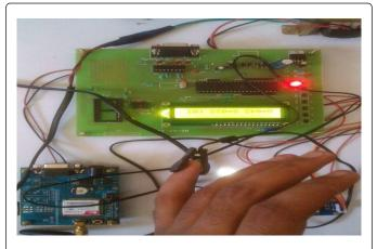
Figure 3: Hardware model of GSM based non-invasive glucose monitoring system.
