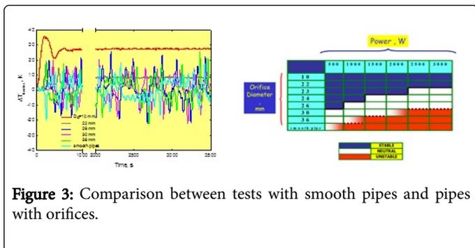
Figure 3: Comparison between tests with smooth pipes and pipes with orifices.
