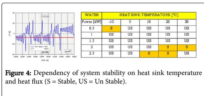
Figure 4: Dependency of system stability on heat sink temperature and heat flux (S = Stable, US = Un Stable).
