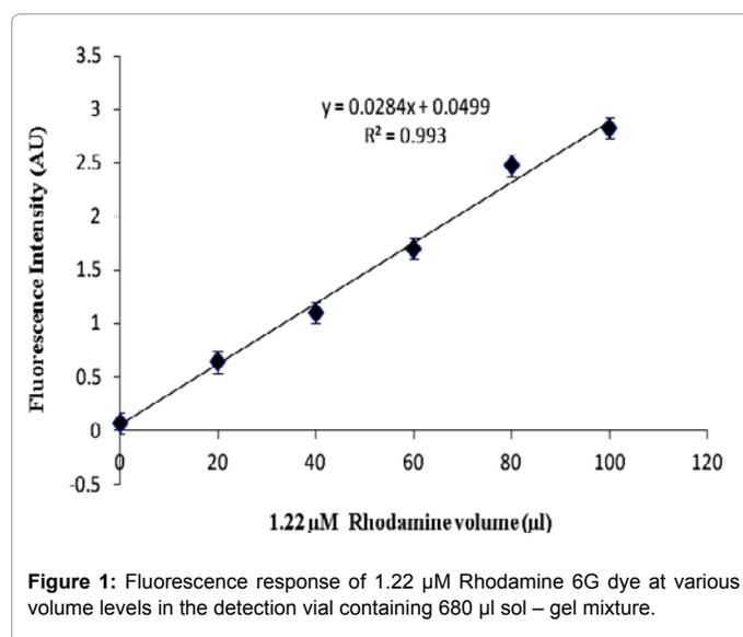
Figure 1: Fluorescence response of 1.22 µM Rhodamine 6G dye at various volume levels in the detection vial containing 680 µl sol – gel mixture.
