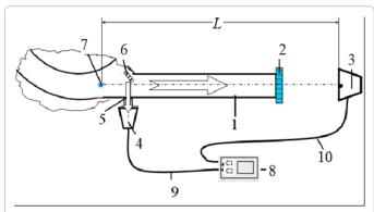
**Figure 2:** Proposed schematic of the measurements: (1) radiation output channel; (2) output window; (3) radiation detector of the measuring channel; (4) detector of the reference channel; (5) reference radiation output channel; (6) mirror of the reference channel output; (7) point of emission of an electron from a stationary orbit; (8) two-beam oscilloscope; (9) reference channel cable; (10) measuring channel cable.
