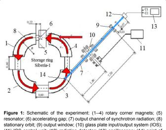
(11) IOS control unit; (12) radiation detector; (13) oscilloscope; (14) point of emission. The distances are given in meters.
