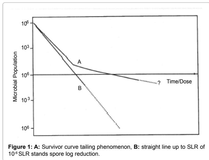
Figure 1: A: Survivor curve tailing phenomenon, B: straight line up to SLR of 10<sup>6</sup> SLR stands spore log reduction.
