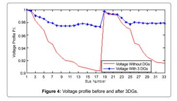
and after the placement of 1 DG, 2 DGs and 3 DGs for 33-bus test system.
