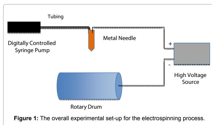
Figure 1: The overall experimental set-up for the electrospinning process.
