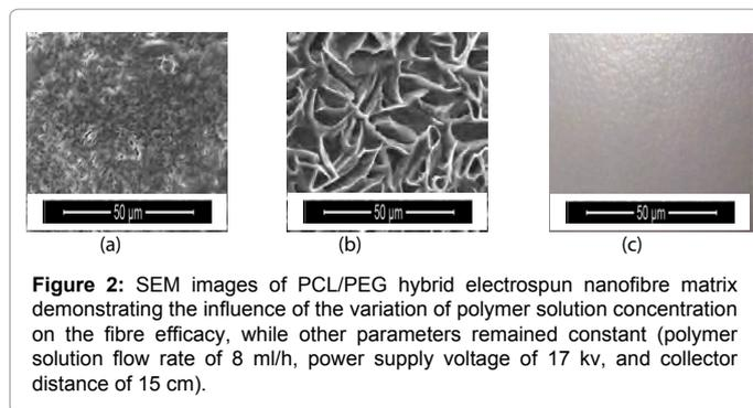
be due to very high surface tension at the tip of the Taylor cone, which could not be opposed by the applied electric potential. Thus, there were no traces of polymers onto the collector (Figure 2c). Therefore, the optimum polymer concentration was considered to be of 20 wt% of PCL/PEG (i.e., 10 wt% of PCL and PEG each component) in dichloromethane. This optimum PCL/PEG polymer solution concentration was used throughout the study.
