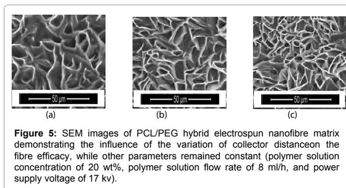
**Figure 5:** SEM images of PCL/PEG hybrid electrospun nanofibre matrix demonstrating the influence of the variation of collector distance on the fibre efficacy, while other parameters remained constant (polymer solution concentration of 20 wt%, polymer solution flow rate of 8 ml/h, and power supply voltage of 17 kv).
