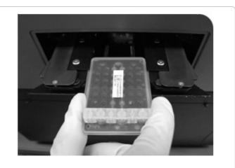
**Figure 1:** A low cost, fully automated, user-friendly, lab on a chip genotyping analysis system (TPSA-003) predicting the risk of rashes by identifying DNA polymorphism markers (HLA-B\*3505) that indicate a high correlation with the risk of drug rash occurrence, which is a side effect of the antiretroviral therapy, nevirapine.
