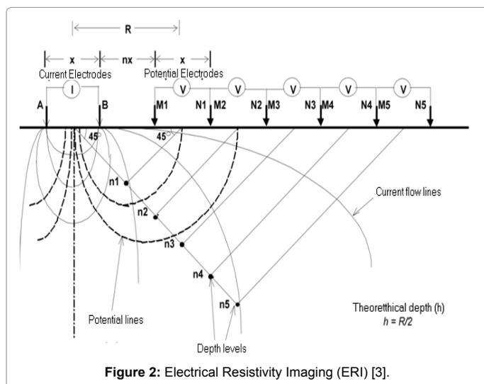
Figure 2: Electrical Resistivity Imaging (ERI) [3].
