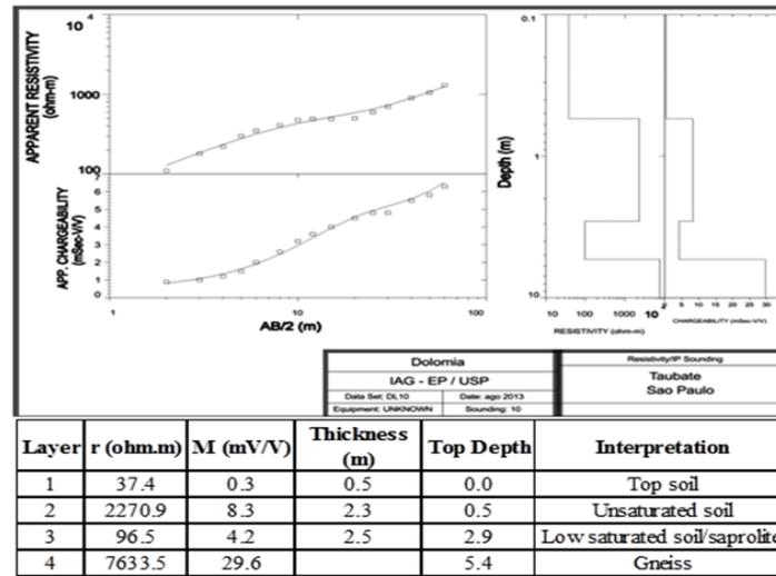
Figure 4: VES10 of the geoelectric model.
