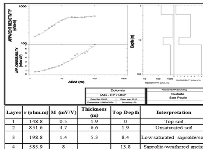
Figure 5: VES05 of the geoelectric model.
