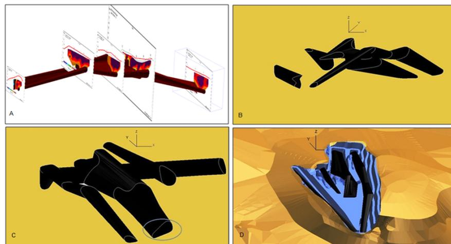
Figure 12: A) Position of ERI profiles; B, C) Geological model; and D) Conceptual pit design.
