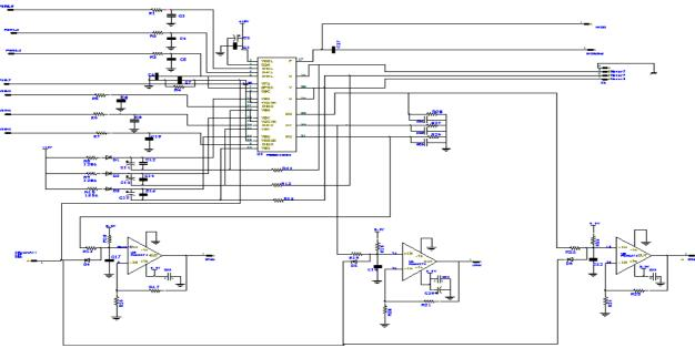
Figure 6: Schematic design of the Smart Power Module
