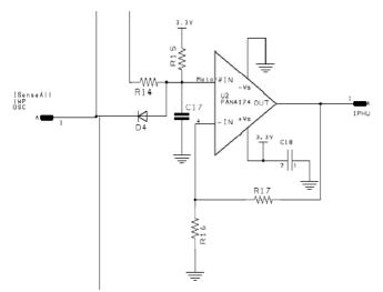
Figure 10: Schematic diagram of Current Sense Circuit
