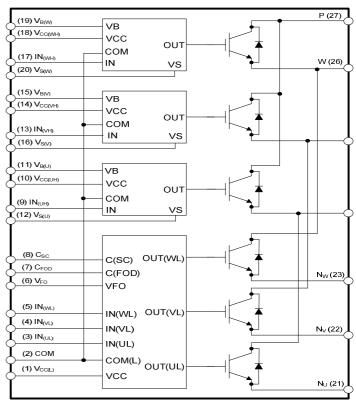
Figure 9: Inner Schematic of FSBS15CH60
