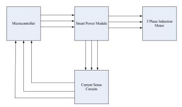
Figure 7: Block Diagram of the flow of Smart Power Module
