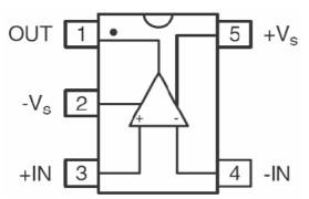
Figure 2: Pin Configuration of FAN 4174IS5X SOT23 [5]
