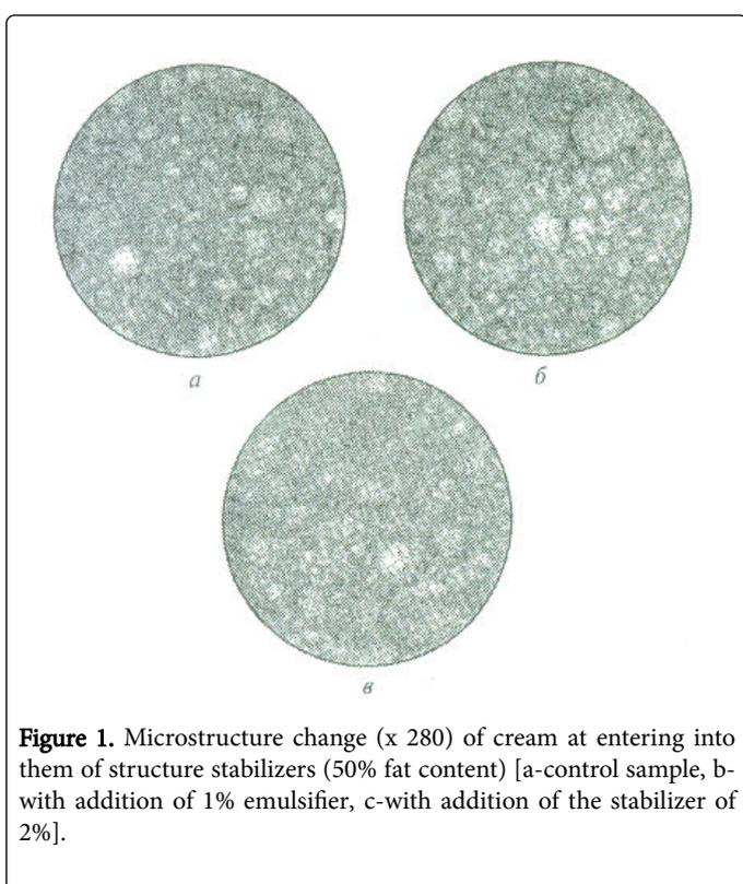
**Figure 1.** Microstructure change (x 280) of cream at entering into them of structure stabilizers (50% fat content) [a-control sample, b-with addition of 1% emulsifier, c-with addition of the stabilizer of 2%].
