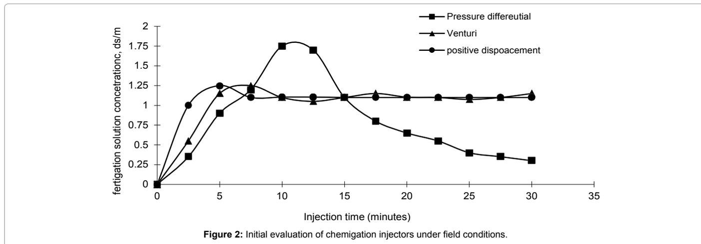
Figure 2: Initial evaluation of chemigation injectors under field conditions.
