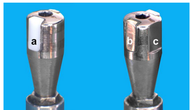
Figure 2: Modified healing abutments with a zirconia sample (a), a gold sample (b) and a polished titanium surface (c).
