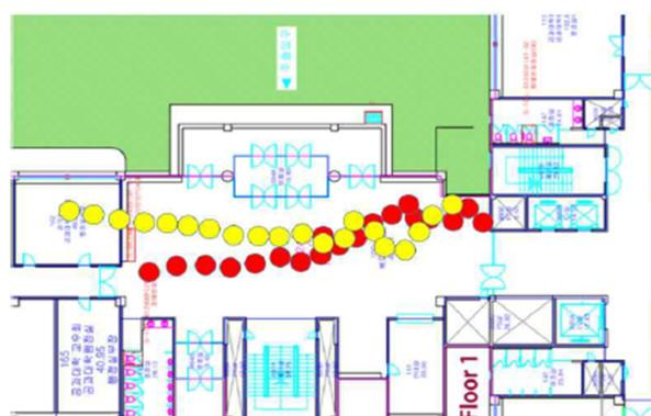
Figure 19: Test result of Inv-FP with PDR in the Engineering test bed from 0 to 40 steps (colored in red circles) and from 200 to 240 steps (colored in yellow circles) in the Engineering test bed.
