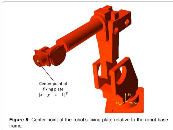
Figure 5: Center point of the robot's fixing plate relative to the robot base frame.
