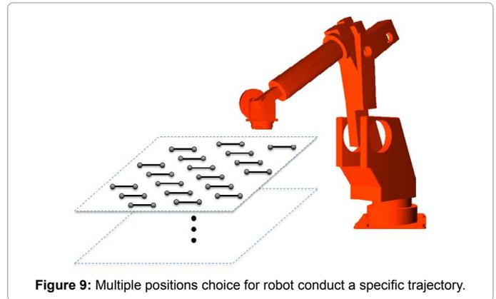
Figure 9: Multiple positions choice for robot conduct a specific trajectory.
