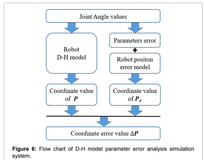
Figure 6: Flow chart of D-H model parameter error analysis simulation system.
