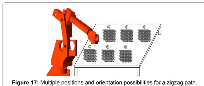
z range is from 800 to 1400. Thus there are 45 testing cube areas within robot working envelope, as shown in Figure 18. The dimension of deposition zigzag path is  $10\text{ mm} \times 10\text{ mm} \times 1\text{ mm}$ , the layer thickness is  $0.1\text{ mm}$ , track width is  $2\text{ mm}$  and overlap is  $0.3$ .
