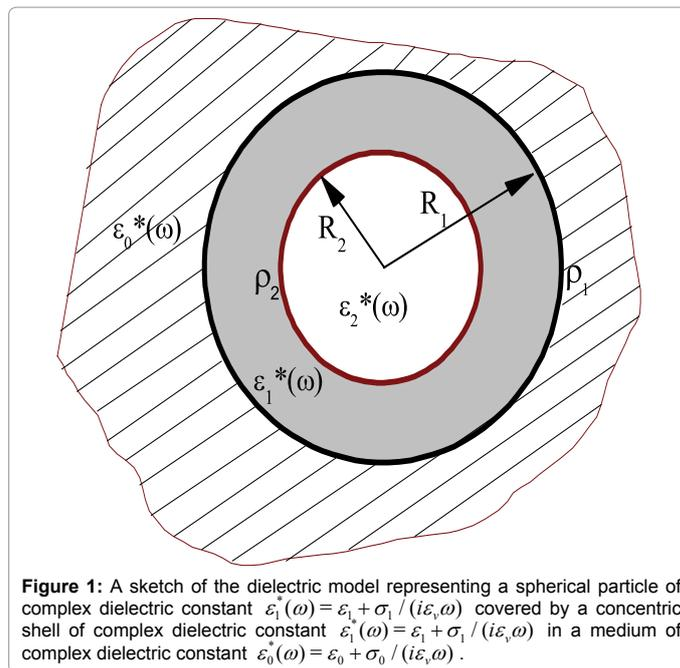
Figure 1: A sketch of the dielectric model representing a spherical particle of complex dielectric constant  $\varepsilon_1^*(\omega) = \varepsilon_1 + \sigma_1 / (i\varepsilon_1\omega)$  covered by a concentric shell of complex dielectric constant  $\varepsilon_2^*(\omega) = \varepsilon_2 + \sigma_2 / (i\varepsilon_2\omega)$  in a medium of complex dielectric constant  $\varepsilon_0^*(\omega) = \varepsilon_0 + \sigma_0 / (i\varepsilon_0\omega)$ .
