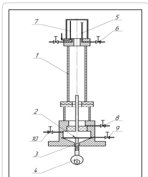
1—a glass tube with 80 mm diameter and 120 mm length, 2—pulsator, made in the form of a membrane, 3—rod, 4—cam, 5—stabilizer, 7—air duct, 6,8,9,10—locking elements
