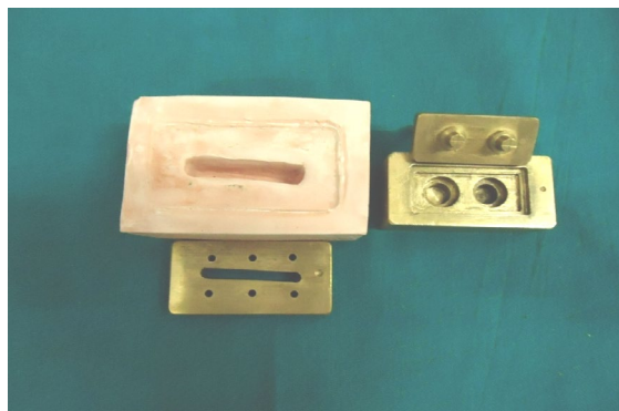
Figure 3: Die stone slab, brass master die, brass custom tray, brass index.
