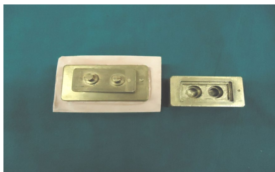
Figure 4: Brass master die stabilized on brass index and die stone slab, Brass Custom tray.
