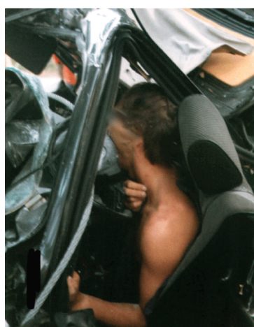
Figure 17: Example of dislocation of the steering column after frontal car collision, accident year 1991.
