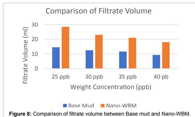
Figure 8: Comparison of filtrate volume between Base mud and Nano-WBM.
