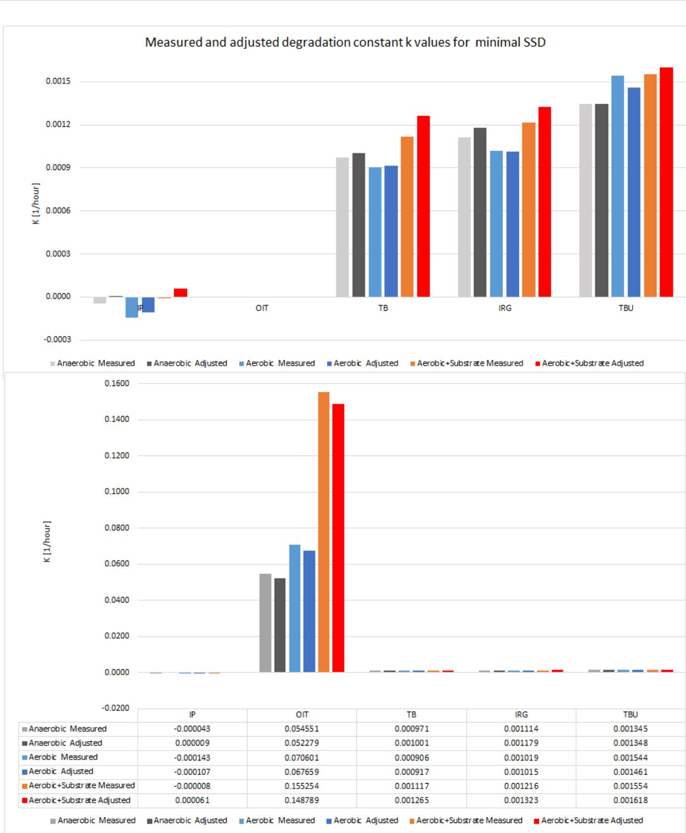
Figure 3: Measured and adjusted degradation constant (h<sup>-1</sup>) for minimal standard square deviation.
