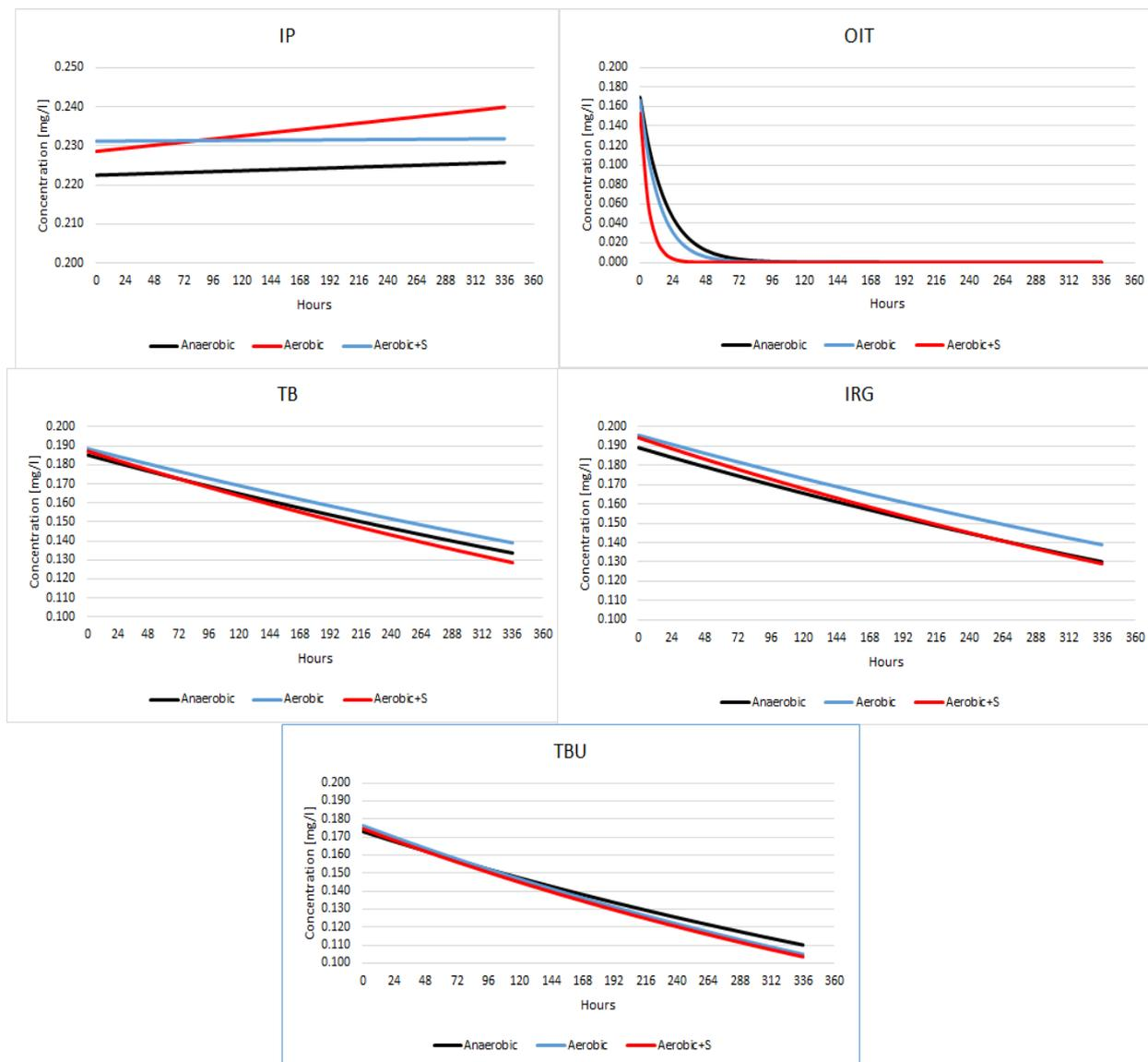
Figure 2: Modeled biocide biodegradation curve by using calculated  $k$  ( $h^{-1}$ ); S=substrate.
