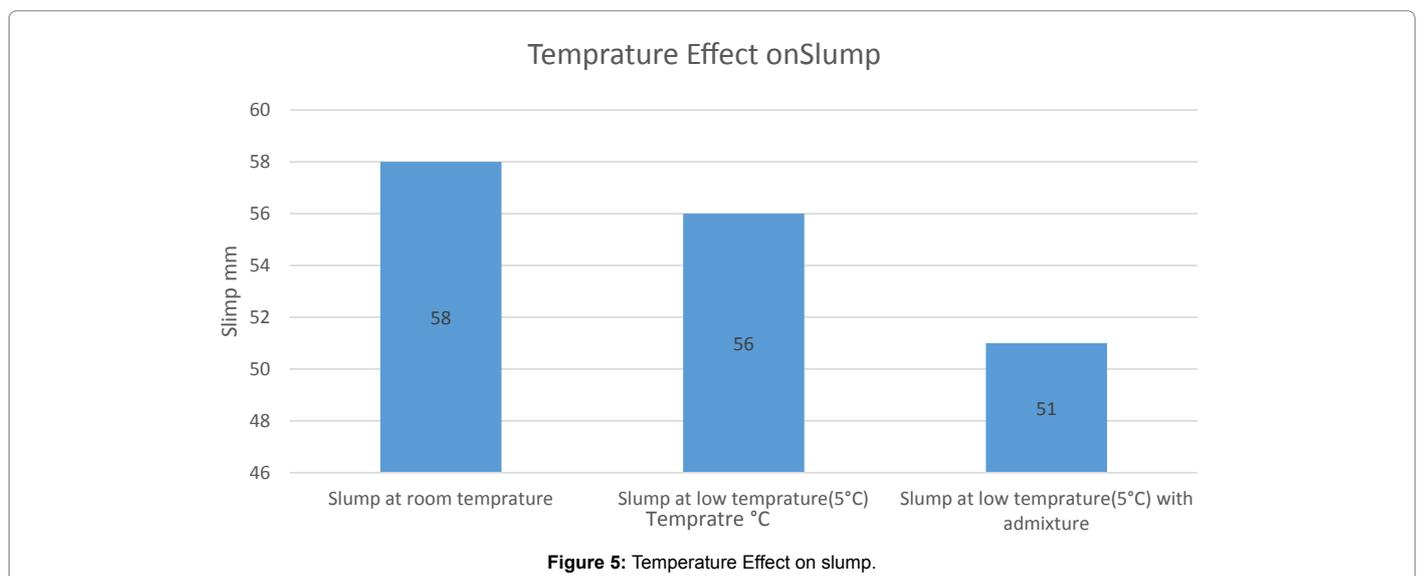
Figure 5: Temperature Effect on slump.
