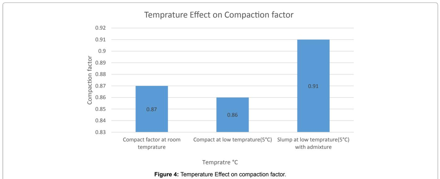
Figure 4: Temperature Effect on compaction factor.
