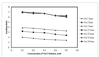
Figure 3: Effect of various concentration of NaCl solution on swelling ratio of PVA hydrogel with 0.3% citric acid at 25 kGy radiation dose.
