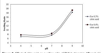
Figure 8: Effect of citric acid on swelling ratio of PVA hydrogel in different pH buffer solution at 25 kGy radiation dose.
